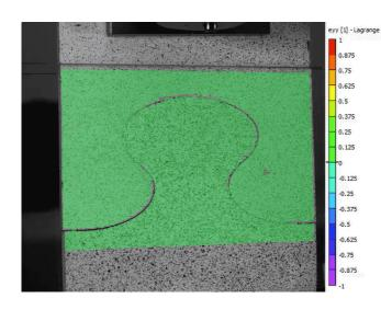
The diabolical ironclad beetle has puzzle piece-like blades in its abdomen that "delaminate" to prevent the beetle's exoskeleton from suddenly failing under immense force. Purdue researchers simulated this mechanism using 3D-printed versions of the blades. Credit: Purdue University/Maryam Hosseini and Pablo Zavattieri
